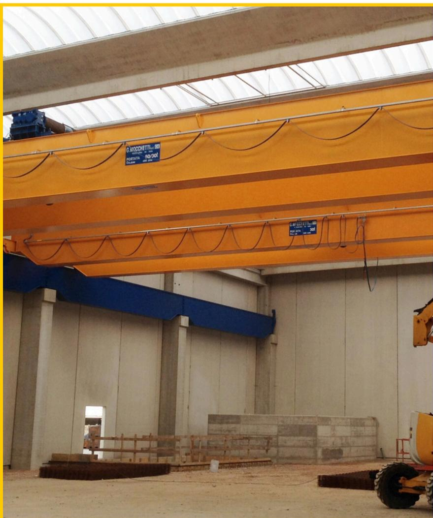
*standard cranes offer control via push-button panel, radio remote control or cabin and speed regulation through inverters.*
