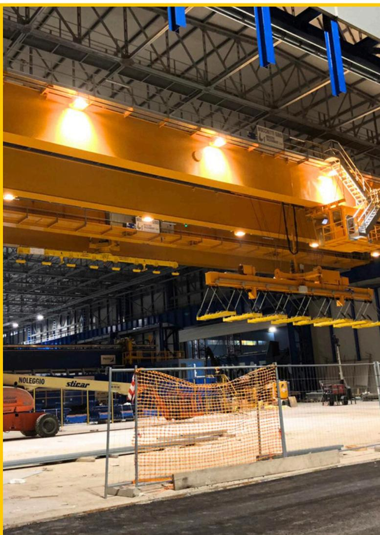
*Automatic cranes are designed to meet the needs of the most demanding customers, leveraging sophisticated software and technologies. These systems, managed via PLC (Programmable Logic Controller), offer high reliability and the ability to operate autonomously, either partially or fully, enabling repetitive load handling without the direct supervision of an operator.*
